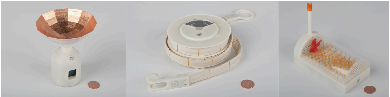
Figure 1. The Weather Stations are three small sensing devices (for purposes of scale, these are shown here next to a UK two pence piece): The Light Collector (LC) displays the ambient light in the home as a continuously updating colour palette. The Temperature Tape (TT) reveals thermal gradients along a thermochromic printed ribbon while the temperature difference between two points – the hook and the eye – is displayed on a dial in the central spool. The Wind Tunnel (WT) senses micro drafts and emulates them over a miniature landscape. For clarity, we present each device separately in this essay though in reality they were developed concurrently. This is a curated rather than chronological account of their production. (The detail in these images is best viewed onscreen from the PDF or the Flickr album found at http://tinyurl.com/attn2detail )
