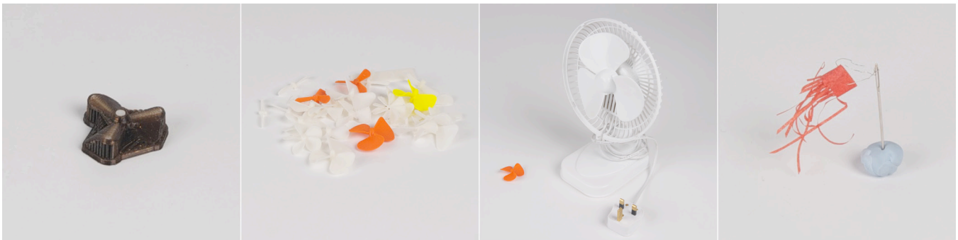
Figure 17. The first image shows a 3D printed propeller fan still enclosed in the support structure used in the machine's build process. This is one of a series of fans designed, printed and tested to find one that would achieve the most disruptive airflow. The final design was influenced by the blades of a conventional desk fan, which seemed to buffet the air the most (therefore producing the dramatic effect on the landscape). The image on the far right shows a miniature wind sock attached to a very small sewing needle, just one of the many props built to place in the landscape. Through this making we developed a greater understanding of crafting wind-catching elements from paper and how small drafts could be visually amplified.
