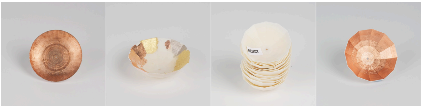
Figure 9. The funnel transformed during a number of iterations to fine-tune a variety of details. The testing of metal leaf and its various finishes and application methods was carried out in conjunction with the development of the LC to optimise the impact of the reflections of the facets. The aim was to achieve a result whereby the funnel acts as a light sensor in its own right, each facet becoming an individual light switch. Simulated tests were completed in CAD software to explore the reflection of the facets so as to ‘funnel’ the light towards the mounted sensor whilst echoing the ambient light on the copper surface. Production methods continually evolved, an initial attempt to print the funnels in a stack over a holiday period failed as the support material between funnels compromised the surface to be leafed. Production funnels had to be printed individually, each taking 11 hours, necessitating the careful management of a printing schedule to avoid any downtime of the 3D printer.
