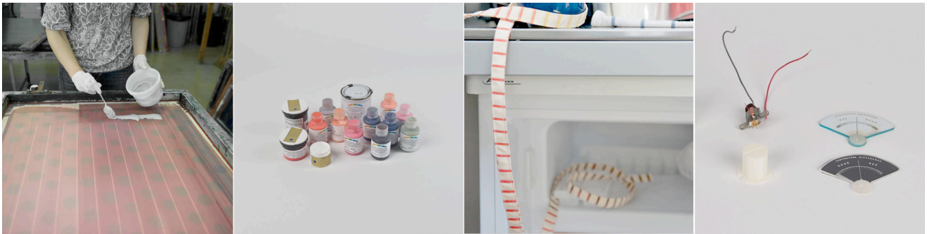
Figure 14. We commissioned a set of bespoke thermochromic pigments to cater for the temperature thresholds that we were interested in. This enabled us to develop a novel layered application of this ink that gave the behaviour of stripes changing colour from black-red-orange-yellow with the ambient temperature of the room. The pigment was silk screen-printed onto calico fabric before being cut up and fed through a bias-binding maker and sewn together to house the sensor cable to create the temperature tape ribbon. Production samples were tested in extreme environments. Other important design decisions concerned the housing of the difference dial and the dial cover. Laser etching tests were carried out to achieve precise depths to make the dial graphics most legible. The dial increments were spaced at a non-linear scale to create more differentiation when the dial needle swings further towards one extreme. Engineering issues were also resolved - bespoke washers were made to account for slight differences in the hand-made panel meter to ensure an accurate fit into the 3D printed casing.
