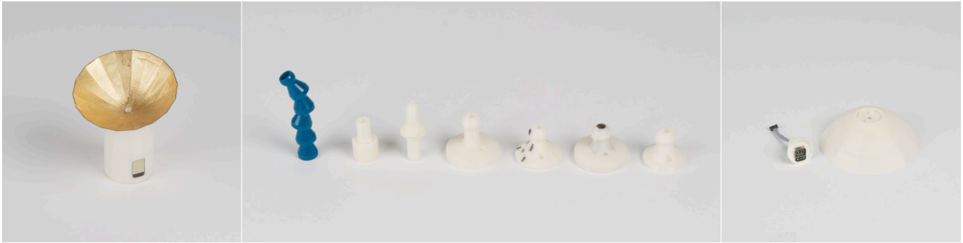
Figure 7. As well as iterating the design to finalise the proportions of the funnel and display window, there were a number of technical and engineering challenges to house the hardware. Having sole use of a 3D ABS printer allowed us to develop a bespoke articulated ball and socket joint (patent pending) to connect the body and the funnel, house the wiring for the light sensor and to produce a greater movement of the funnel, similar to an angle-poise lamp (allowing directional sensing). We were also keen for the copper leafing to have an uninterrupted finish inside the funnel (bar a small window onto the sensor) and this necessitated the development of a fairly complex hidden housing on the underside. Again the ability to print custom parts gave us the freedom to devise a method for installing the RGB sensor without mechanical fixings, making it possible to hide the part within the walls of the funnel.
