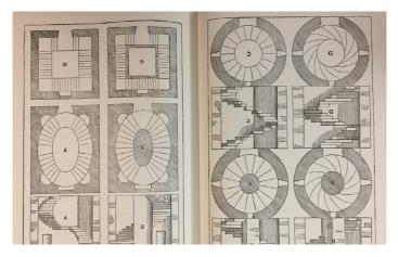
Types of staircases: spiral, oval and straight. Palladio described how and when to use each type; for example, spiral staircases are suited for "very restricted locations because they take up less space than straight stairs but are more difficult to go up."
