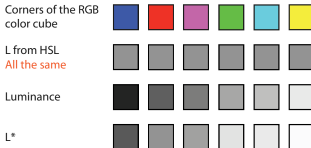
Figure 10.3. Comparing HSL lightness, true luminance, and perceptually linear luminance L^* for six colors. The computed HSL lightness L is the same for all of these colors, showing the limitations of that color system. The true luminance values of these same six colors, as could be measured with an instrument. The computed perceptually linear luminance L^* of these colors is the best match with what we see. After [Stone 06].
